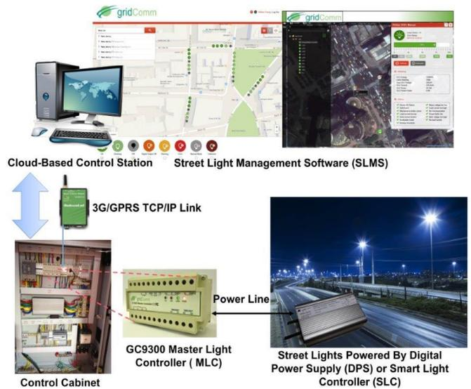
**Figure 1 gridComm SLMS System Architecture**
